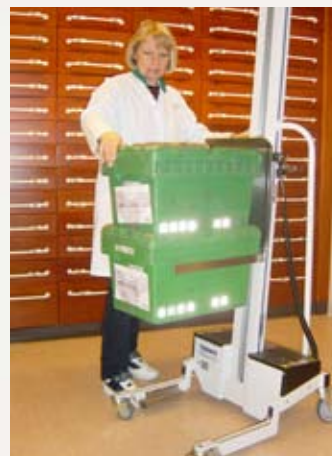
Crates in stacks are handled with a fork tool on PRO70.
